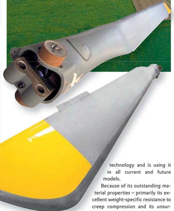
anium, the life cycle of these structures is four to five times longer, because no material fatigue occurs," says Denecke. With the help of sandwich technology, therefore, operating periods of 15,000 hours or 40 years – the maximum service life of a helicopter – can be reached. This is why Eurocopter is committed to this
