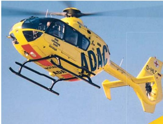
The rotor blades of helicopters are subject to enormous stresses. At a travel speed of 250 kilometers per hour, the rotor of a helicopter like the EC145 rotates 400 times per minute. This means the tips are moving at speeds of about 220 m/sec. The centrifugal forces this creates can reach about 1,000 times the force of gravity.
