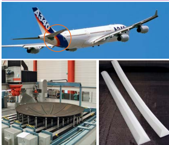
1 | Airbus A340-600, rear pressure bulkhead (left), CNC-machined and net-shape-thermoformed ROHACELL® A-profiles (right)
