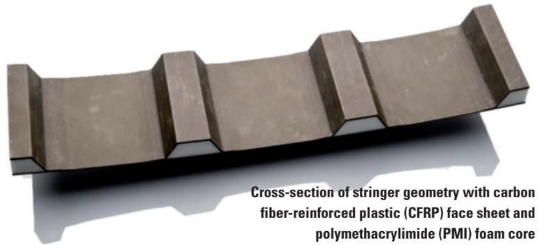
Cross-section of stringer geometry with carbon fiber-reinforced plastic (CFRP) face sheet and poly(methyl methacrylate) (PMI) foam core
