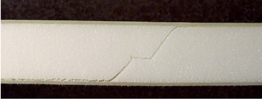
Picture 2: Fatigue fracture of PMI 51 S, P/P_{crit}=65\% , n=1.1 \cdot 10^6 cycles
