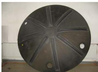
The rear pressure bulkhead, the first large size composite prototype on C919, was rolled out in October, of which structure ROHACELL® is used as the stringers to enhance the stiffness and buckling properties of the part.
