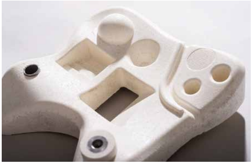
Fig. 1. The demonstration component contains, by way of example, two different inserts and shows possible geometries with a defined surface structure that can be achieved with the newly developed PMI foam
